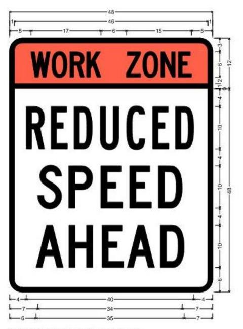
3" Radius, 1" Border, Black on Fluorescent orange; "WORK", C 2K 60% spacing; "ZONE", C 2K 60% spacing;
